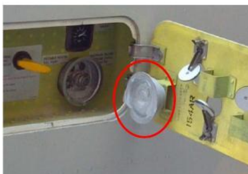
Figure 3-2: Example of ice accumulation on fill fitting (Potable water service panel)
