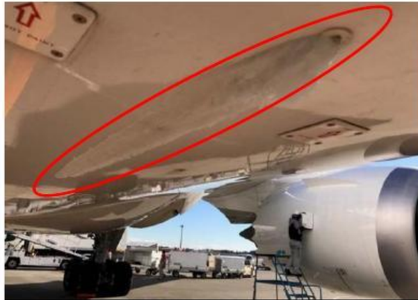
Figure 3-3: Example of ice accumulation on fuselage drain
