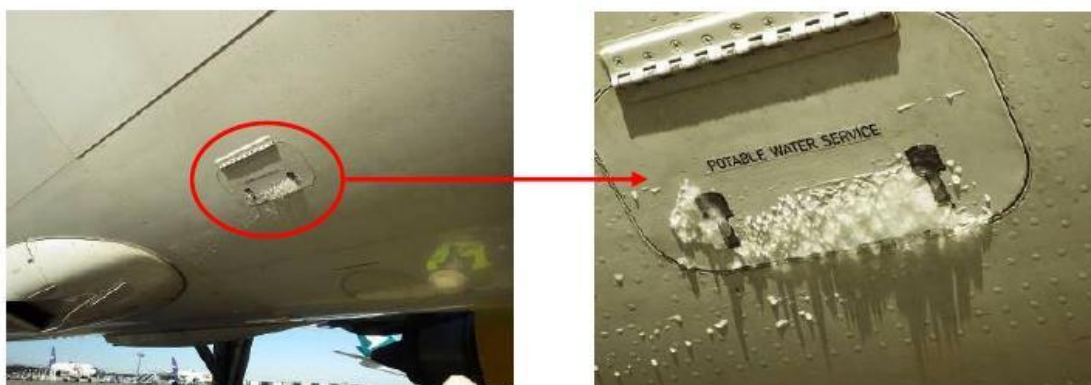
Figure 3-1: Example of ice accumulation on potable water service panel
